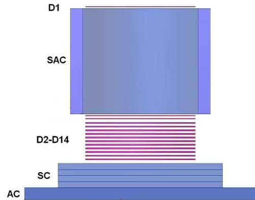
(b) The physical scheme of one detecting stack.
