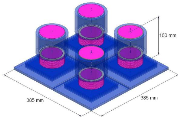
(a) The structure of whole spectrometer-telescope.
