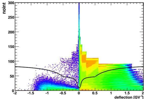
Fig. 2: Distribution of the *noint* variable, correlated to the shower starting point in the calorimeter. Particles above the black lines are selected as (anti)proton candidates.
