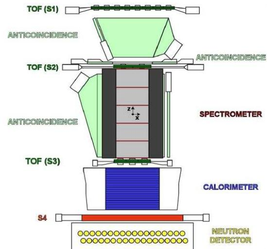
Fig. 1: Schematic drawing of the PAMELA apparatus, showing sensitive areas of the various subdetectors to scale, in a longitudinal section. The right-handed coordinate system used in the experiment is also represented.
