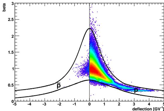
Fig. 4: The velocity ( $\beta$ ) versus deflection distribution, obtained after having applied the tracker selection, the charge selection performed with the ToF and the tracker, and the calorimeter selection. Particles within the black lines are selected as (anti)proton candidates.
