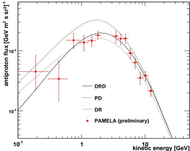
Fig. 5: The antiproton flux measured with the PAMELA instrument. Predictions from some theoretical models describing pure secondary  $\bar{p}$  production [8] are also shown for comparison: i) a plain diffusion model with an ad-hoc break in the diffusion coefficient (PD); ii) a distributed re-acceleration and power-law diffusion with no breaks (DR); iii) a new self-consistent model of diffusive re-acceleration with damping (DRD).
