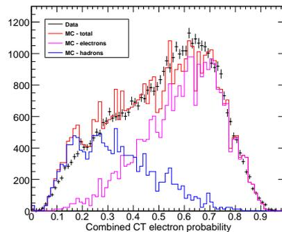
Fig. 2: Electron probability from the Classification Tree output. LAT data are compared with on orbit background model for events above 100 GeV. The selection on all the other quantities is already applied.
