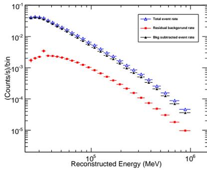
Fig. 3: The residual background rate (in red) is evaluated, for each energy bin, using the on-orbit environment simulation and is subtracted from the measured LAT event rate (in blue). The resulting rate (in black) is deconvolved with instrument response functions to provide the electron spectrum.
