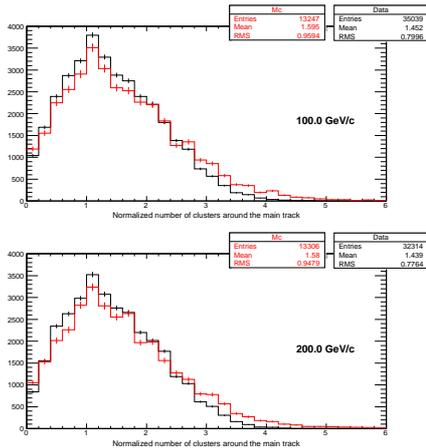
Fig. 1: Number of hits around the best track (normalized to the track length) for a normal incidence electron beam at 100 GeV/c (top plot) and 200 GeV/c (bottom plot). CU data in black and the corresponding MC simulation in red.
