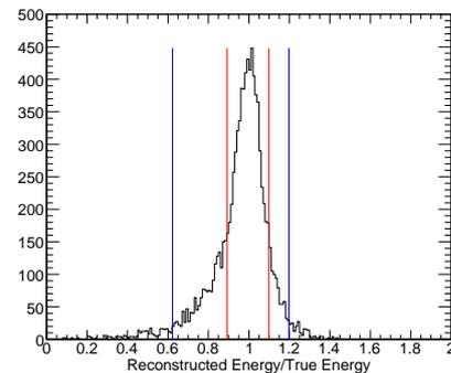
Fig. 5: This figure shows how the energy resolution is evaluated using the electron simulation. For each bin in true energy (from  $\sim 562$  GeV to  $\sim 767$  GeV in this case) the distribution of the reconstructed energy divided by the true energy is plotted. The vertical red lines show the boundaries of the 68% containment window (for a resolution of 20%) and the blue lines are the boundaries of the 95% containment window.
