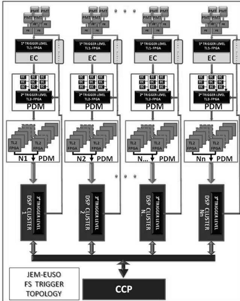
Fig. 1. Structural scheme of the different levels of trigger.
