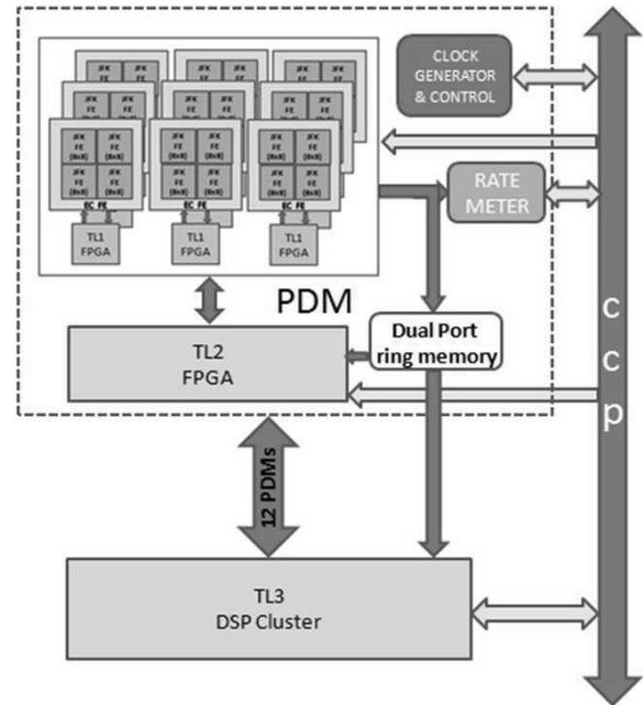
Fig. 2. Block diagram of the FS PDM electronics. In this case 12 PDMs are connected to one of the Digital Signal Processor (DSP) cluster.
