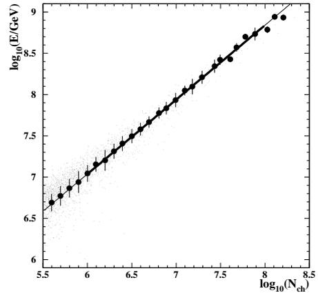
Fig. 2: Scatter plot of  $E$  vs  $N_{ch}$  for iron primary nuclei. See fig. 1 for detailed explanation of the meaning of dots and error bars. The fit is used to obtain the parameters  $a$  and  $b$  of expression 1.
