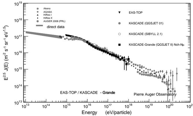
Fig. 6: All primaries energy spectrum (intensity multiplied by  $E^{2.5}$ ) obtained with KASCADE-Grande data applying the  $N_{ch} - N_{\mu}$  technique. A comparison with other experimental results is also presented.
