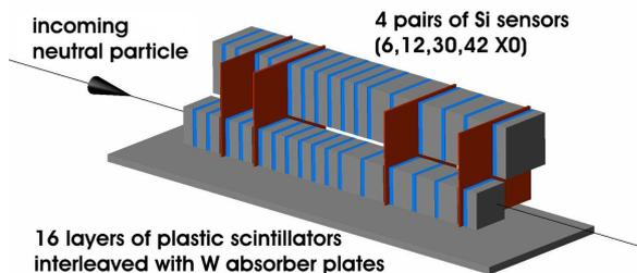
Fig. 1: Schematic drawing of the LHCf Arm2 calorimeter. The two towers are 24 cm long and have transverse dimensions of  $2.5 \times 2.5 \text{ cm}^2$  and  $3.2 \times 3.2 \text{ cm}^2$ .
