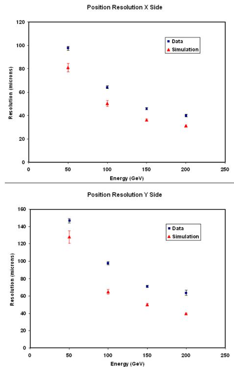
Fig. 5: X and Y position resolution, on the first Si module, for electromagnetic showers as a function of incident electron energy.
