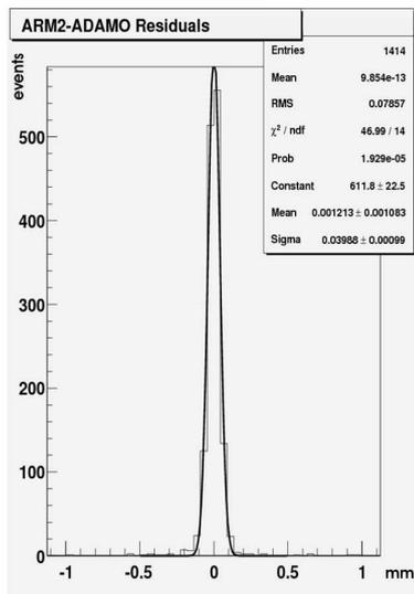
Fig. 4: Distribution of residuals for the shower centre X coordinate in the first Si module, referred to the extrapolated ADAMO telescope track. Data taken for 200 GeV electrons.
