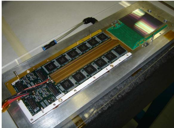
Fig. 2: Open view of one side of a Si detector module. On the left: two FE half-hybrid boards (6 PACE3 chips each) with the central area occupied by kapton fan-outs; on the right: the Si sensor, glued on the fiberglass pitch adapter.
