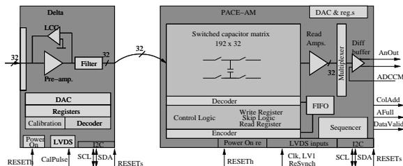
Fig. 3: Functional block scheme of PACE3 chip.
