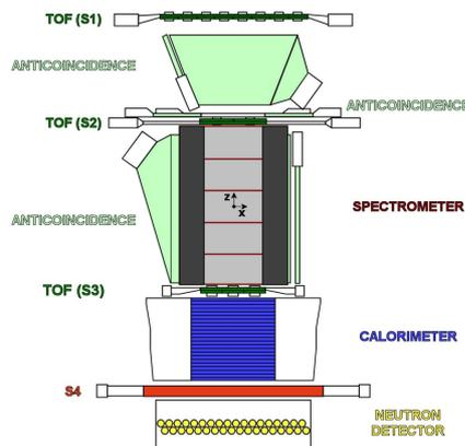
Fig. 1: A schematic view of the PAMELA apparatus.
