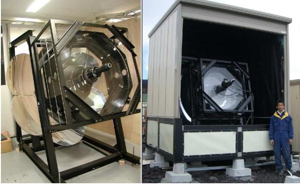
Fig. 1: The Ashra detector (for lower elevation FOV). The right was taken after mounting the components.
