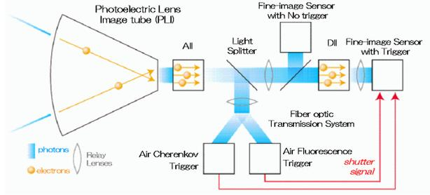
Fig. 2: Conceptual figure of ‘Image Pipeline’ and ‘Trigger and Readout’. Light collected by Optical System is incident from the left [22].
