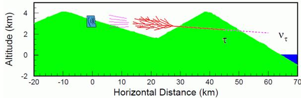
Fig. 3: Conceptual figure of this observation (the Earth-skimming neutrino detection technique). The right mountain is Mauna Kea and the left is Mauna Loa.
