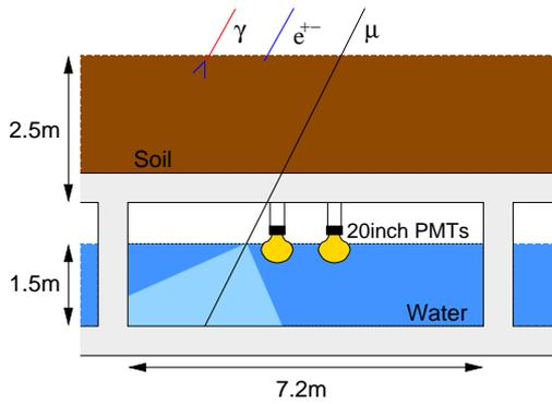
Fig. 1. Schematic side view of the Tibet MD array. Each muon detector is set up 2.5 m underground and has a waterproof concrete pool, 7.2 m wide  $\times$  7.2 m long  $\times$  1.5 m deep in size, equipped with two 20 inch-in-diameter PMT (HAMAMATSU R3600).
