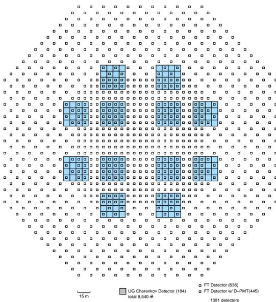
Fig. 2. Schematic view of the Tibet AS+MD array for the MC simulation. The open squares show 0.5 m<sup>2</sup> plastic scintillation detectors which composed Tibet AS array. This array is extended to 8,3000 m<sup>2</sup> from the present array (3,7000m<sup>2</sup>). The filled squares show the proposed 52 m<sup>2</sup> water Cherenkov detector cells of the Tibet MD array buried 2.5 m underground.
