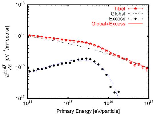
Fig. 2. All-particle spectrum around the knee. Solid line is the global component calculated by present model. Dashed line is the fit to the excess component seen in Tibet 3 data[11] which can be approximated as  $f_x(E) \propto E^{-2} \exp(-E/4\text{PeV})$ . The dot-chained line is the sum of the global component and  $f_x(E)$
