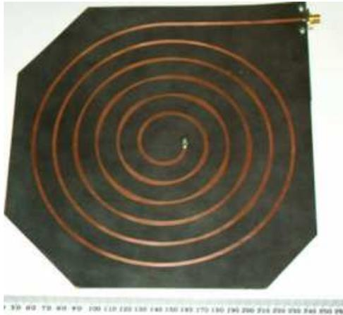
Fig. 2. Photograph of our prototype dedispersion filter. The spiral shape is for compactness only – the dedispersion is achieved by varying the waveguide width.
