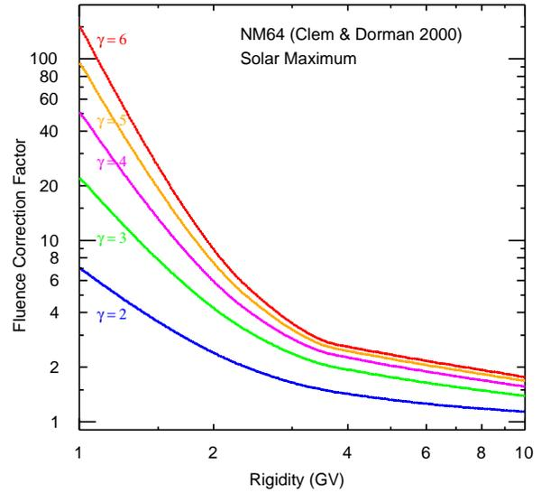
Fig. 2: Correction factor vs. rigidity for various solar proton spectral index values, using the NM64 yield function [15] and the 1990 solar-maximum GCR proton spectrum [12].
