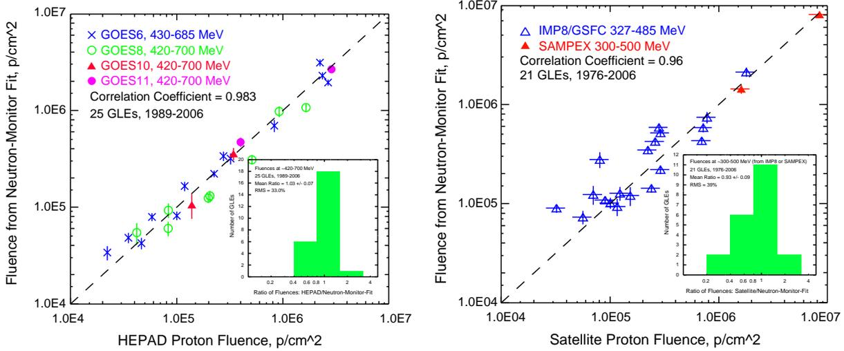
Fig. 5: Correlation of proton fluences from our NM analyses versus corresponding values from GOES/HEPAD (left) and from IMP8 or SAMPEX (right). Insets show histograms of the ratios of satellite-fluences to NM-fluences.
