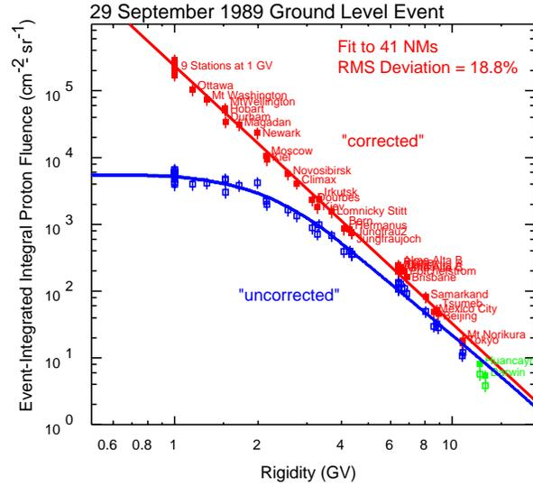
Fig. 4: NM fluences before and after correction in the 1989-Sep-29 GLE.
