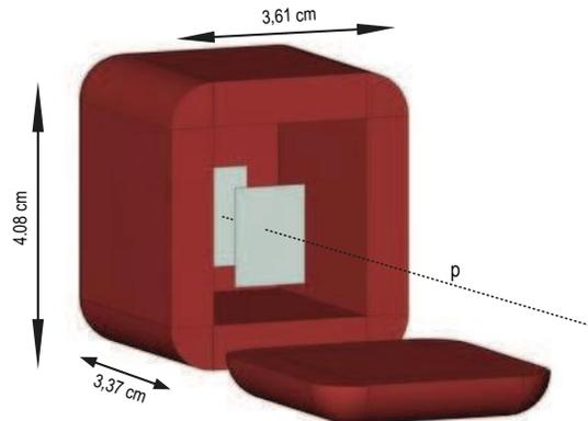
Fig. 1. LISA-PF radiation monitor set-up. Silicon wafers are sketched inside the shielding copper box. An incident proton trajectory is shown. Other details are reported in the text.
