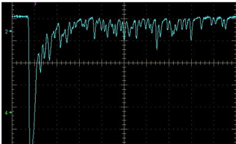
Fig. 2: Oscilloscope trace of a single event. The timescale is 80ns/div (800ns full trace). Each of the small peaks in the tail are consistent with single photoelectron signals.
