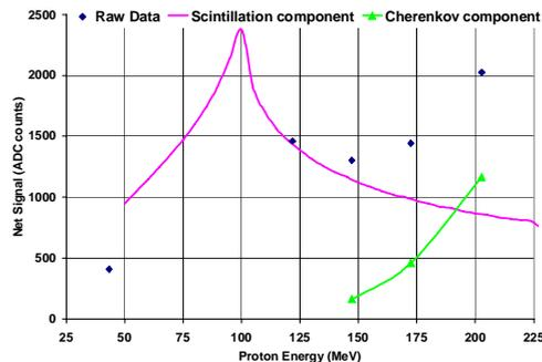
Fig. 5: Raw data and analysis results for the CZ detector exposed to protons at 50, 125, 150, 175 and 205 MeV. The two curves show the scintillation and Cherenkov components of the total signal separately.
