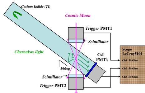
Fig. 3: Experimental setup for CsI to detect muons. The angle between the CsI principal axis and the average muon trajectory is  $56^\circ$ .
