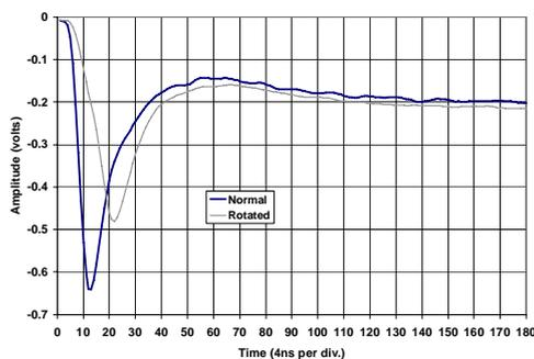
Fig. 6: Average response for muons in the CsI. The two peaks are due to Cherenkov photons directly incident on the PMT and those reflected from the far end of the CsI log. The long tail shows the delayed response of the primary scintillation. The two traces are for different setups (see text). The timescale is 4ns/div (73 ns full trace).
