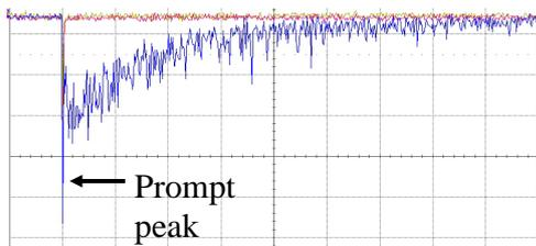
Fig. 4: Oscilloscope trace of a muon generated signal in CsI. The timescale is 500 ns/div. The large prompt peak is due to Cherenkov photons.
