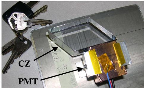
Fig. 1: CZ detector with PMT.
