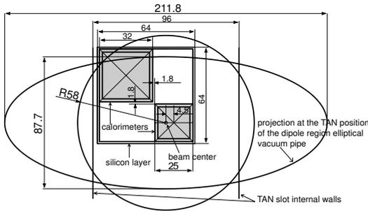
Fig. 3: Cross section of detector 2. Grey squares indicates the calorimeter in the detectors while green square shows the coverage of the silicon strip sensor.
