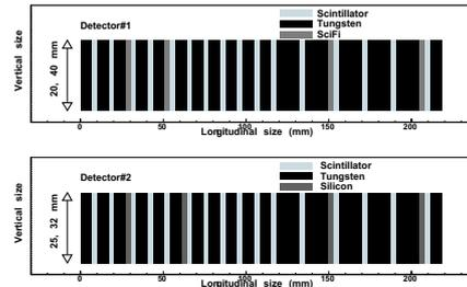
Fig. 1: Longitudinal structure of detector 1(top) and detector 2(bottom); grey, light blue, orange and red indicate the layers of tungsten, plastic scintillator, SciFi and silicon strip sensor, respectively.
