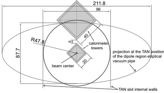
Fig. 2: Cross section of detector 1. Grey squares indicates the calorimeter in the detectors. Vertical and elliptical blue lines indicate the physical aperture limited by the walls of the TAN and the beam pipe respectively.
