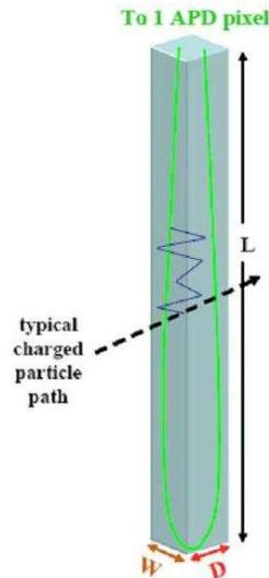
Fig. 1. A PVC cell containing liquid scintillator and wavelength shifting fiber. A charged particle incident on the front face produces light that bounces off the cell walls until absorbed by the fiber. The fiber routes the light to an APD.
