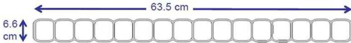
Fig. 3. Cross section of the NOνA extrusion, made of PVC plastic.
