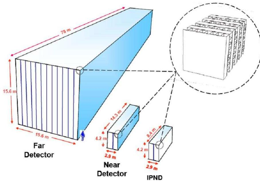
Fig. 4. A schematic of the three NOνA detectors
