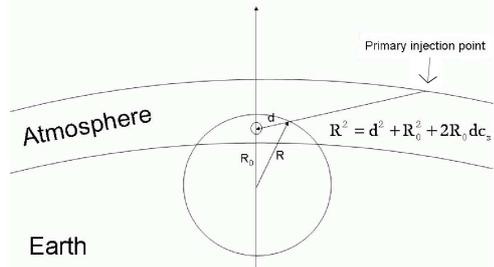
Fig. 1. Sketch of the sampling procedure for underground sites. Once the primary direction is sampled, a rock sphere is created around the experimental hall with a radius  $R$  equal to the corresponding amount of rock that has to be crossed to reach the underground site. This value is read from the map location. The primary direction is then traced back to the upper atmosphere, thus locating the primary injection point.
