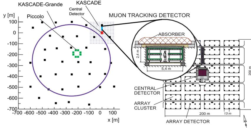
Fig. 1: Layout of the KASCADE-Grande experiment distributed over the Research Center Karlsruhe. KASCADE is situated in the North-East corner of the Center: note the position of the Muon Tracking Detector.
