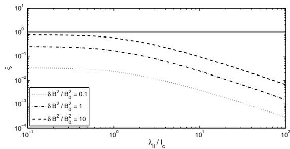
Fig. 3. The scattering anisotropy  $\xi = \kappa_{\perp}/\kappa_{\parallel}$  versus the ratio  $\lambda_{\parallel}/l_c$  for different values of  $\delta B^2/B_0^2$ . The solid line corresponds to isotropic scattering  $\xi = 1$ .
