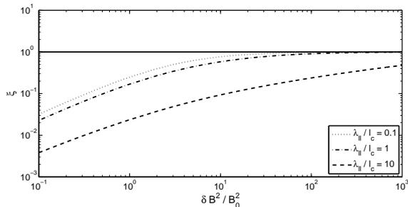
Fig. 4. The scattering anisotropy  $\xi = \kappa_{\perp}/\kappa_{\parallel}$  versus the ratio  $\delta B^2/B_0^2$  for different values of  $\lambda_{\parallel}/l_c$ . The solid line corresponds to isotropic scattering  $\xi = 1$ .
