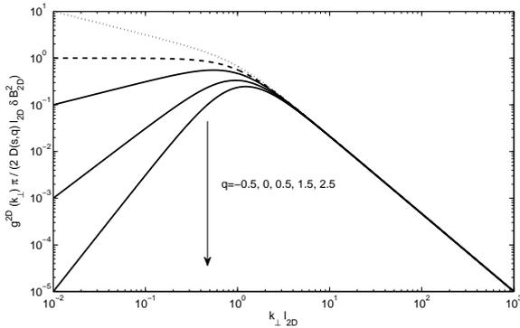
Fig. 1. The turbulence spectrum of the two-dimensional modes for different values of the energy range spectral index  $q$ . For  $q = 0$  we have a constant spectrum, for  $q < 0$  a decreasing spectrum, and for  $q > 0$  an increasing spectrum in the energy range.
