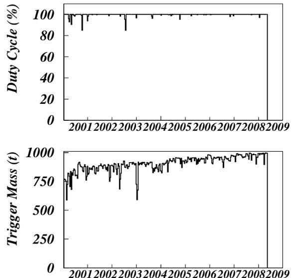
Fig. 1: LVD duty cycle (top) and trigger mass (bottom) during 2001-2009.
