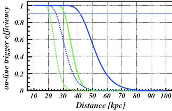
Fig. 4: On-line trigger efficiency versus distance (lower scale) and percentage of SN1987A signal at 10 kpc (upper scale) for  $E_{cut} = 7-10$  MeV (light green and dark blue lines, respectively) and  $M = 330$  t (dotted) and 1000 t (continuous) for LVD stand alone.
