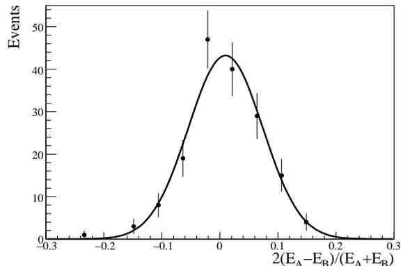
Fig. 5. Relative difference between the energy reconstructed with the two different SD reconstruction procedures A and B, as discussed in the text, for events above  $E = 10^{19}$  eV. The line is a Gaussian fit to the histogram with reduced  $\chi^2$  5.9/10, mean  $0.014 \pm 0.006$  and RMS  $0.068 \pm 0.005$ .
