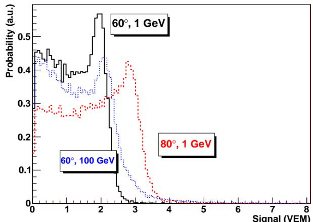
Fig. 1. Surface detector response to inclined muons. Probability of measuring a signal in VEM (vertical equivalent muon) for muons of zenith angle  $60^\circ$  and energy 1 GeV (continuous histogram),  $60^\circ$  and 100 GeV (dotted histogram), and  $80^\circ$  and 1 GeV (dashed histogram).
