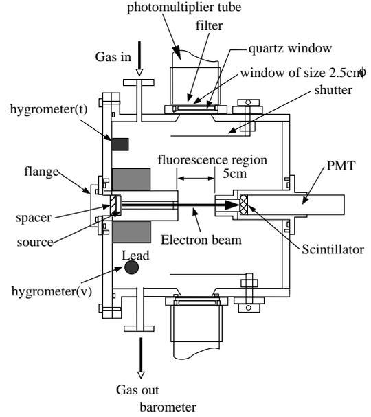
Fig. 1. Top view of the chamber. Laboratory air was passed through water or a desiccant to add or reduce humidity before filling into the chamber, respectively. The resultant humidity was measured by two hygrometers, hygrometer(v) (VAISALA HMP234) and hygrometer(t) (Toplas TA502).
