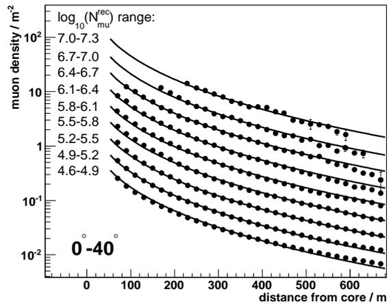
Fig. 3: Measured muon density distribution (dots) for zenith angles  $0^\circ$ – $40^\circ$  and different intervals of the reconstructed muon number. The lateral distribution function of Eq. 3 (curves) with the muon number  $N_\mu$  set to the measured mean muon number  $\bar{N}_\mu^{\text{rec}}$  in each interval describes the data quite well.
