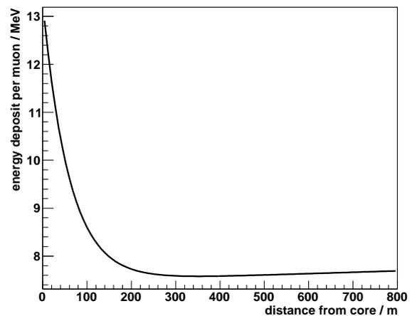
Fig. 2: Average energy deposit per muon in a KASCADE muon detector as a function of the distance of this detector from the shower core (muon LECF according to Eq. 1).
