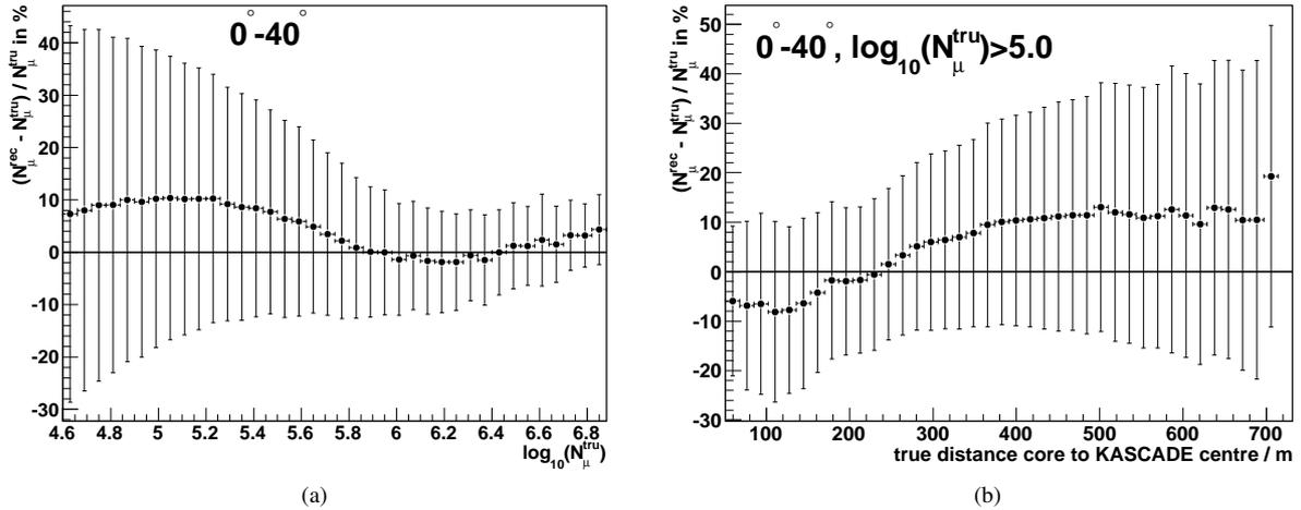
Fig. 4: Reconstruction quality tested based on Monte Carlo simulations. In case *a*) the deviation of the reconstructed to the true muon number is shown as a function of the true muon number, in case *b*) as a function of the distance of the shower core to the centre of the KASCADE array. In both cases the error bars represent the statistical uncertainty (RMS) in a single measurement.
