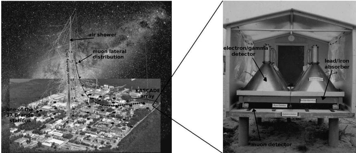
Fig. 1: *Left*: An air shower with the core located in the Grande array. Although the KASCADE detector field is far away from the core, non-zero muon densities can be measured there. *Right*: Detector station of the KASCADE-array equipped with electron/gamma and separate muon detectors.
