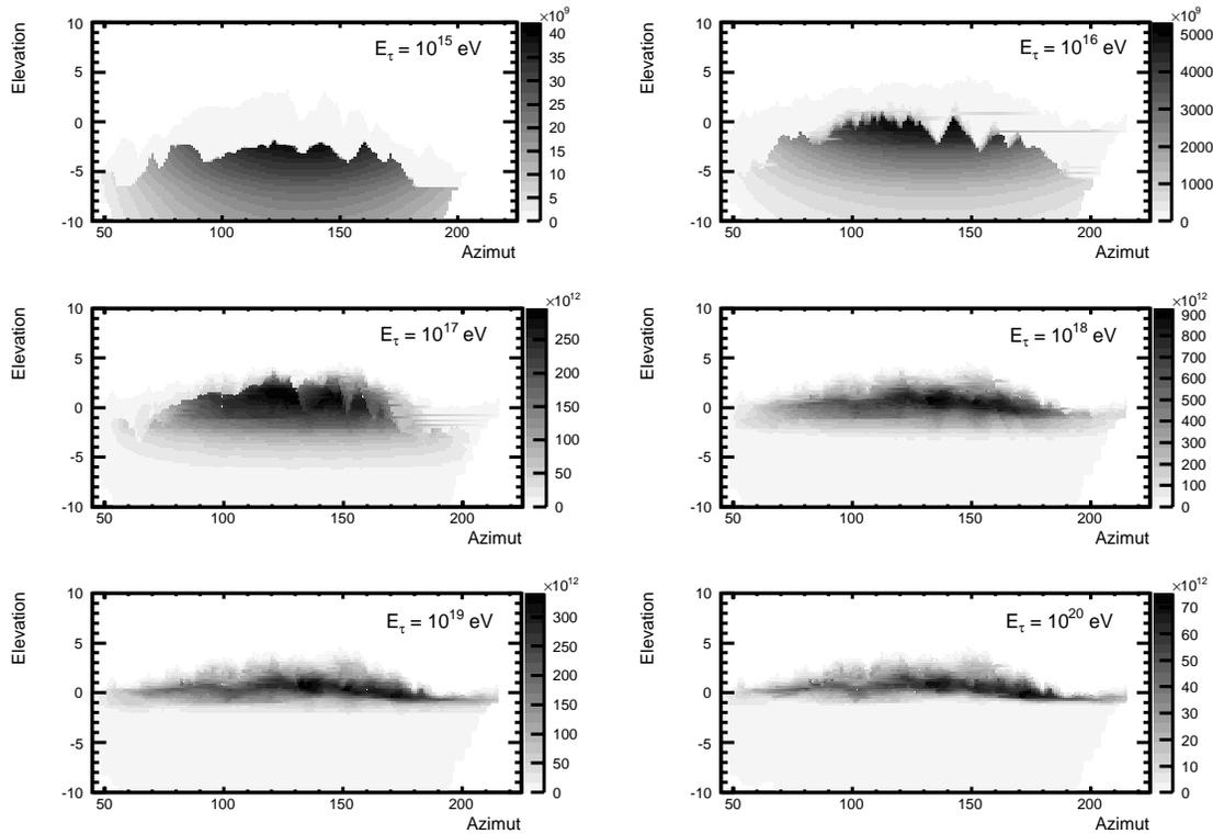
Fig. 1: Neutrino landscape : the sensitivity to  $\nu_\tau$  is computed for each pixel of incoming shower directions taking into account the real mountain topography. The neutrino sensitivity is given in  $\text{cm}^2 \text{s}$  for one year exposure of one cluster and for different neutrino energies. The detector array configuration is the one describe in the text. In these plots, each pixel is  $6.1 \times 10^{-5}$  sr.
