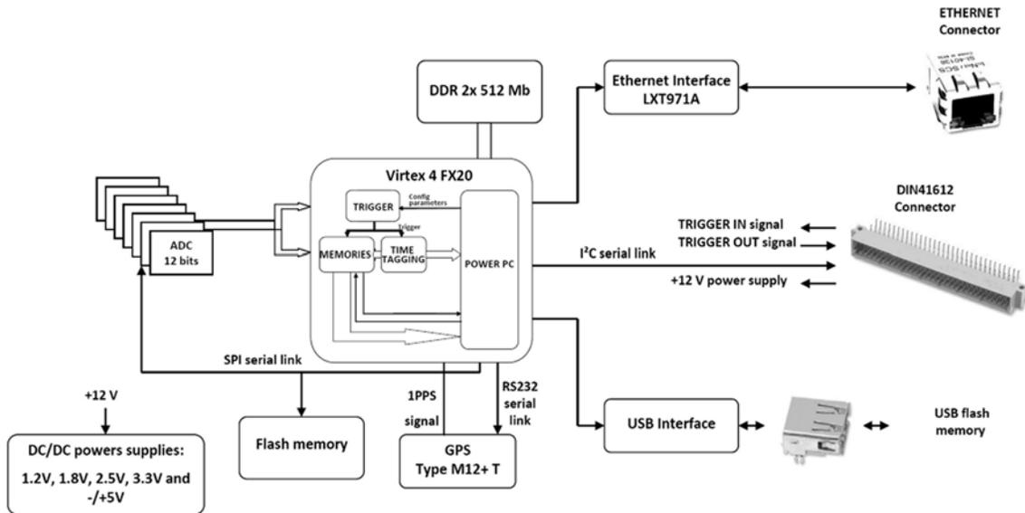
Fig. 3: Schematics of the data acquisition system.
