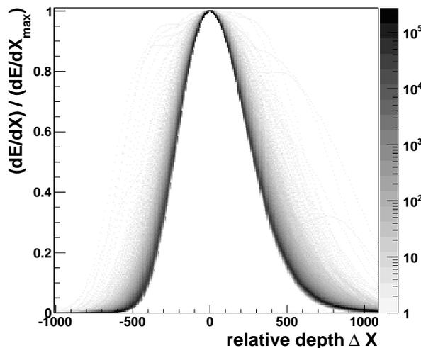
Fig. 1. Superposition of 30000 energy deposit profiles in  $\Delta X$ . The CONEX [10] simulations are for proton primaries. Equal numbers of showers were generated with the QGSJet, QGSJetII.03, and Sibyll interaction models [11]–[13].
