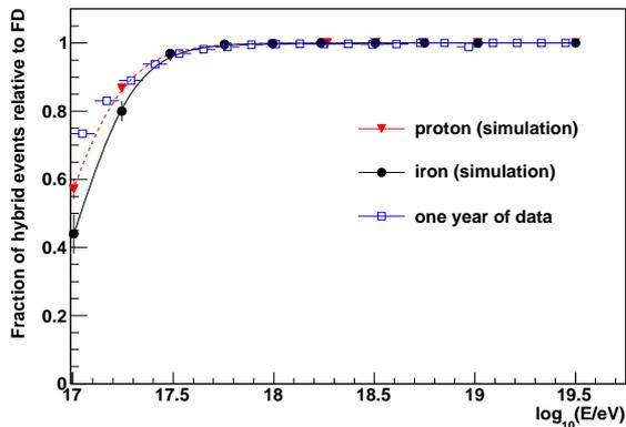
Fig. 2. Relative hybrid trigger efficiency from hybrid simulation for proton, iron and data. All the events are taken for zenith less than  $60^\circ$ .
