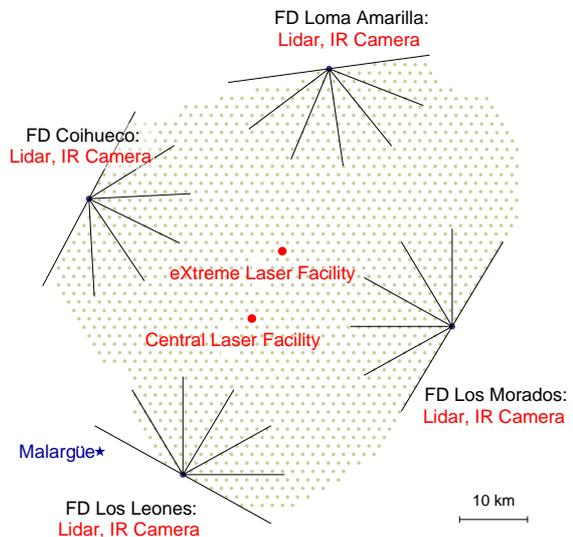
Fig. 1. Atmospheric monitoring devices map
