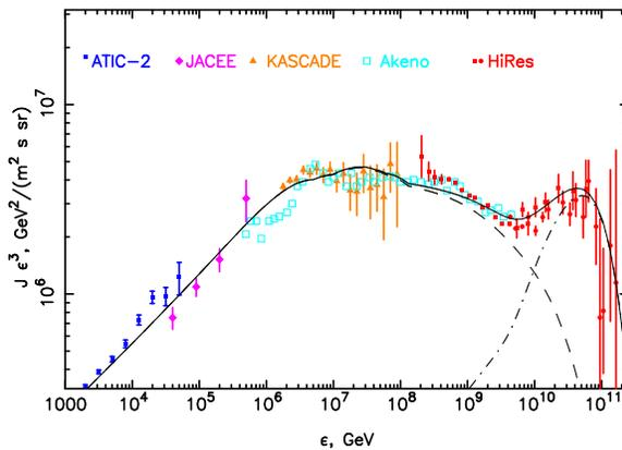
Fig. 3. The same as in Fig.1, but for the ankle scenario. The dashed line represents the Galactic component, which includes CRs produced in SNRs and reaccelerated CRs. The dash-dotted line represents the extragalactic component; it corresponds to the source spectrum  $J_A^s \propto \epsilon^{-2}$  [4].
