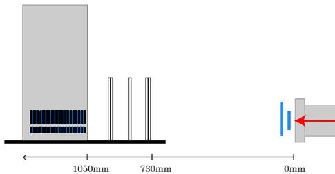
Fig. 1: Setup of the SPS experiment (not in scale). The dark and big rectangles indicate the place of the LHCf calorimeters and their container, respectively. Beam enters from right along the arrow and tagged by two small plastic scintillators. In front of the detector a silicon tracker ADAMO was installed on the movable table together with the LHCf calorimeters.
