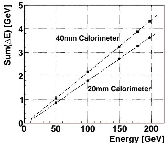
Fig. 4: Linearity of the energy estimator. The summed energy deposits obtained from the experiment (filled marks) and the MC simulation (open marks) are plotted as functions of incident energy. Two series are the results for the 40 mm and the 20 mm calorimeters of the Arm1 detector. Dotted lines are the linear fits of the experimental data.
