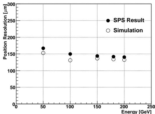
Fig. 5: Position resolution of the Arm1 detector as a function of the incident electron energy. The results for the first X layer are plotted together with the results of MC simulation.
