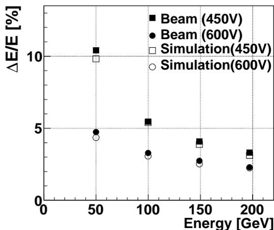
Fig. 3: The energy resolutions of the 25 mm calorimeter as functions of the incident electron energy. Difference in the two PMT gains (450V and 600V) is due to the effect of the pedestal fluctuation measured during the beam test. The results of MC simulation including the pedestal effect are also plotted.
