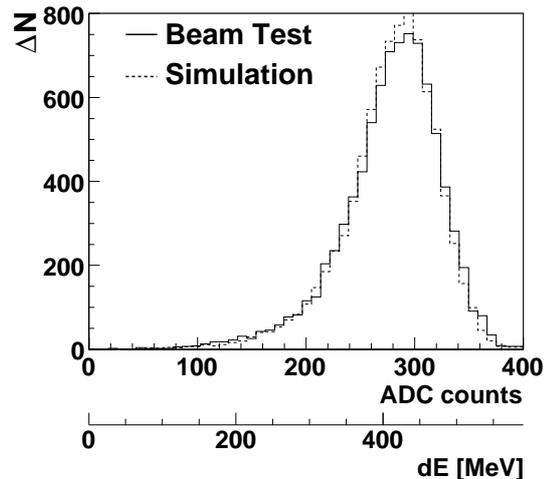
Fig. 2: Comparison of the charge distribution measured by ADC and energy deposit calculated by MC simulation in the 4<sup>th</sup> layer of the calorimeter for 150 GeV electron showers
