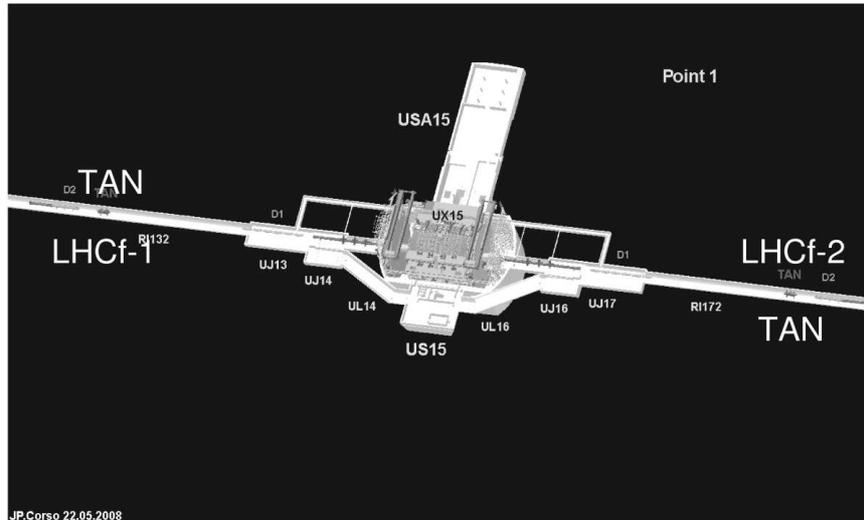
Fig. 1. The layout around the IP1 of LHC. The structure at the center indicates the ATLAS detector surrounding the collision point. The LHCf detectors are installed in the instrumentation slot of the TANs located  $\pm 140$  m from IP1. Two independent detectors, LHCf Arm1 and LHCf Arm2 are installed at either side of IP1.
