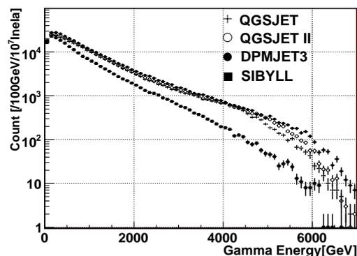
Fig. 4. Expected energy spectrum of gamma-rays measured by one of the LHCf calorimeters. Calculation was performed with four major hadron interaction models used in the cosmic-ray study. The statistical error bars for the operation of  $10^3$  sec at the luminosity of  $10^{29} \text{ cm}^{-2} \text{ s}^{-1}$  are indicated.
