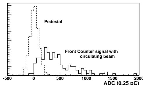
Fig. 5. Beam-gas background observed in one of the LHCf Front Counters during LHC beam commissioning in September 2008. Solid histogram shows the charge distribution of the signal found in the FC faced to the circulating beam while dashed histogram shows pedestal.
