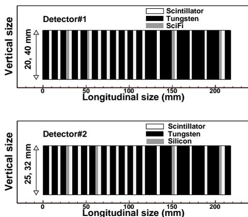
Fig. 3. The longitudinal structure of the LHCf calorimeters. Top (Bottom) panel shows the structure of the Arm1 (2) detector that uses SciFi (Silicon strip detector) as the position sensor.
