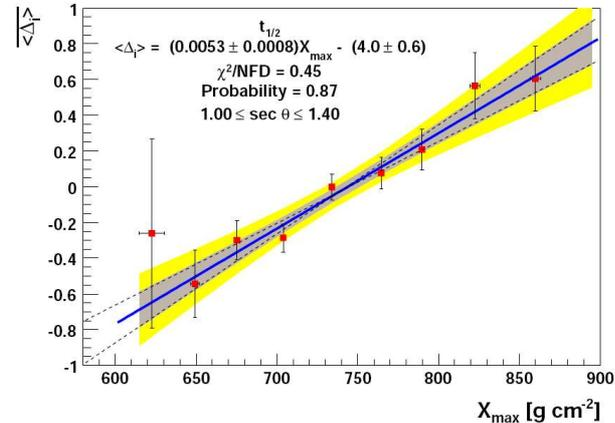
Fig. 3. The average  $\langle \Delta_i \rangle$  as a function of  $X_{\max}$  for selected hybrid events. A correlation is found which is parameterised with a linear fit. The shaded areas show the estimated uncertainty (one and two  $\sigma$ ), obtained by fluctuating each point randomly within the measured error bar and repeating the fitting procedure.
