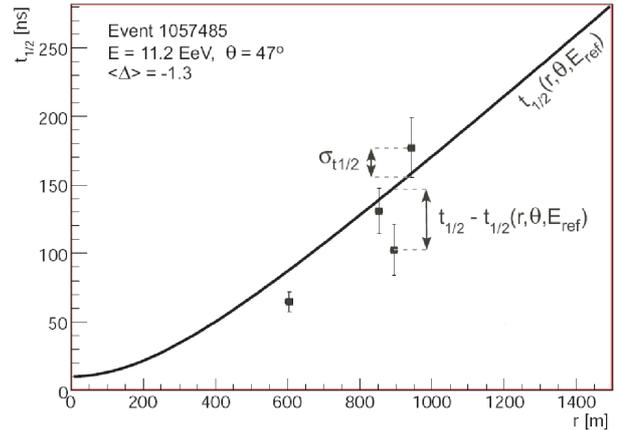
Fig. 1. Risetime vs distance to the core. The curve is the benchmark risetime and the data points represent the measurements of risetime of each detector with uncertainties for this particular event.
