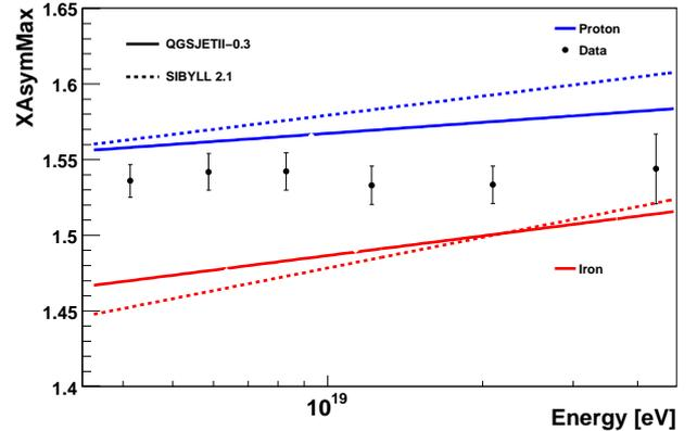
Fig. 5. Position of maximum asymmetry vs. primary energy for different models and primaries. Lines correspond to fitted distributions of MC samples for proton (blue) and iron (red) primaries.
