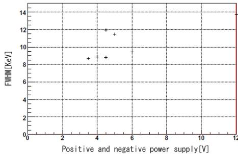
Fig. 7. Resolution of high-gain preamplifier. 59.5 KeV gamma ray was measured with a preamplifier and an S3590.
