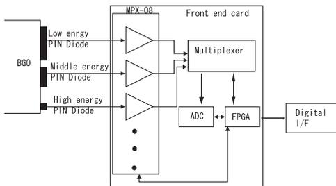
Fig. 5. Block diagram of a read-out system with MPX-08.
