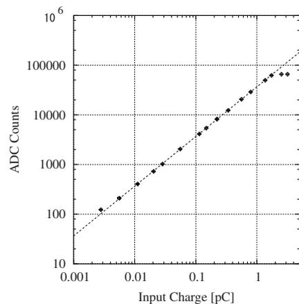
Fig. 3. Linearity of A225 measured by a test pulse. The A225 was operated using a power supply of +12 V.
