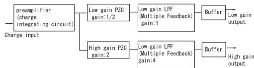
Fig. 9. Block diagram of the internal circuit in a front-end ASIC.
