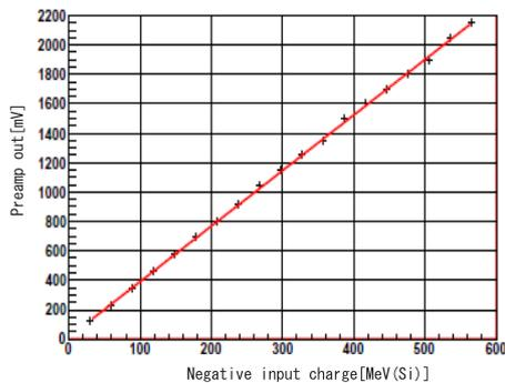
Fig. 8. Linearity of the preamplifier in the new hybrid FEC.
