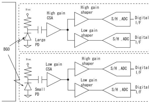
Fig. 6. Block diagram of read-out system using a new hybrid FEC.
