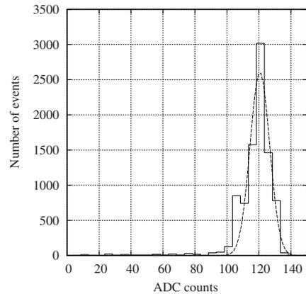
Fig. 2. Energy distribution of 59.5 KeV gamma ray measured with an A225 and a Si-PIN photodiode (Hamamatsu S3589)
