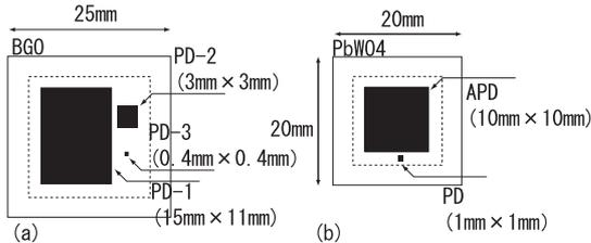
Fig. 1. Design example of photodiode assembly. (a) A three Si PIN-PDs assembly installed on the side of a BGO and (b) an assembly consisting of Si PIN-PD and Si APD installed on a PbWO<sub>4</sub>.
