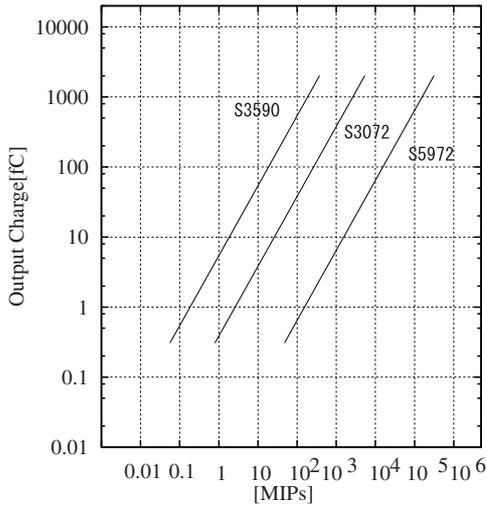
Fig. 4. The expected dynamic range with triple photodiodes and an A225.
