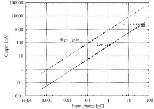
Fig. 10. Linearity of front-end ASIC obtained by SPICE simulation.
