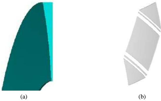
Fig. 1. (a) Detail of the corrector lens in the Geant4 simulation. The curvature of the corrector ring is magnified to be visible. (b) A segment of the telescope mirror. The trapezoids joined to make the mirror element are artificially displaced for better visualization.
