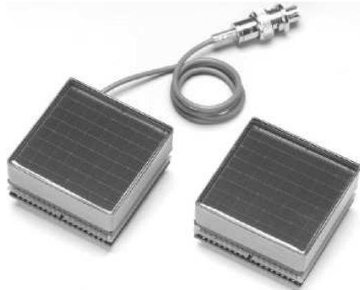
Fig. 2. Hamamatsu H8500 multi-anode photomultipliers.  $8 \times 8$  independent pixels,  $6 \text{ mm} \times 6 \text{ mm}$  each. 12 dynodes. Quantum efficiency  $\approx 25\%$  (for model B).  $HV_{\max} = 1100\text{V}$ . Gain  $10^6$ . Photo and data taken from Hamamatsu publicity material.
